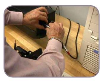
Then, the PMT cables are released by pressing the small lever on the side of each.
