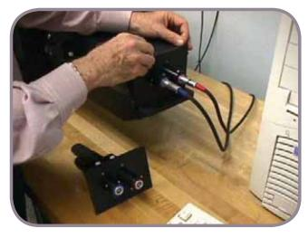
First, the thumbscrews holding the panel in place are removed.
