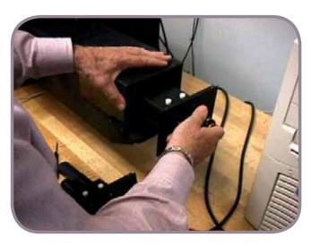
Remove the detector panel as shown. Replace with the new panel by reversing these steps.
