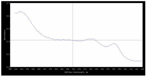
First scan from measurement (above) was subtracted from all subsequent scans, so as to produce the difference spectra, shown below (which show the increasing magnitude of the change, presumably as oxygen was lost to the solvent, PBS):
