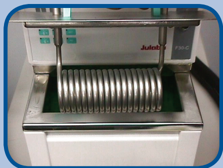
Olis-added circulating coil to preferred water bath.
