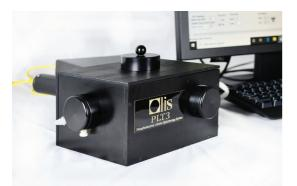
The superior OLIS acquisition scheme is achieved using sophisticated FPGA device and code which contains 100 photon counters which sequentially receive the output of the single photon counting photomultiplier tube detector. Sample excitation is by a computer controlled pulsed LED; detection is by an exquisitely sensitive photon counter.
