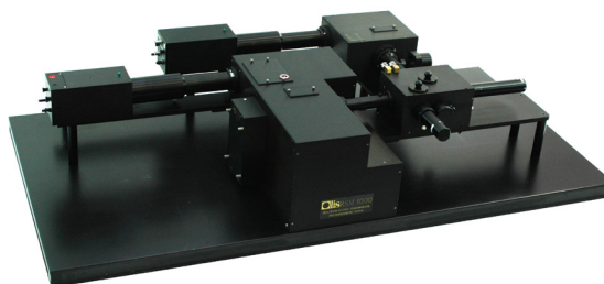
RSM configured for absorbance and fluorescence
